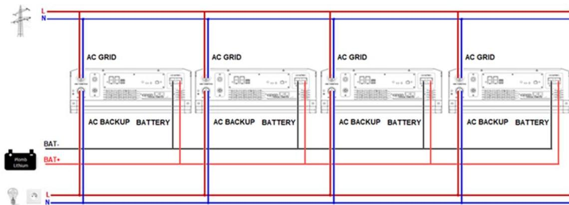
Up to 6 can be connected in parallel on the same installation with a limitation of 100A per phase with the provided SmartMeter.
