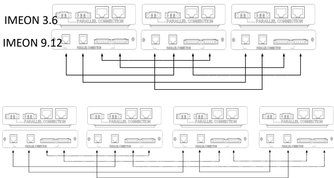
Wiring of parallel plate must be done as above.
